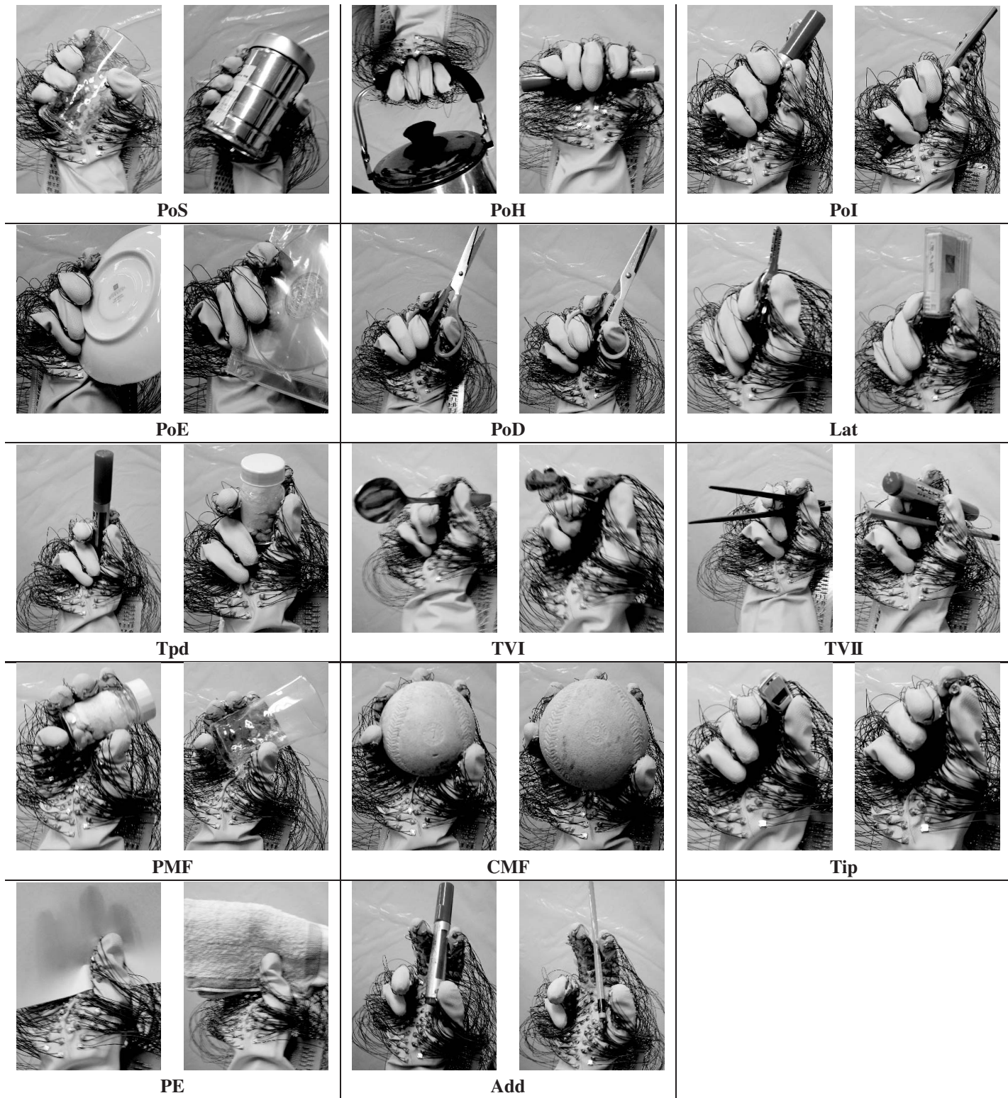
Fig. 6. Appearances of Kamakura's grasp types with the Cyber Glove and the tactile sensing glove.
