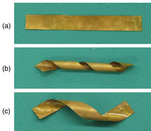
**Figure 4.** IPMC undergoing thermo-mechanically induced shape memory cycle: (a) original shape; (b) programmed shape; (c) recovered shape.
