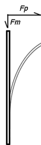
Fig. 3 Illustration of IPMC bending motion and measured force: F_m (measured force element or force element parallel to IPMC) and F_p (force element perpendicular to IPMC).
