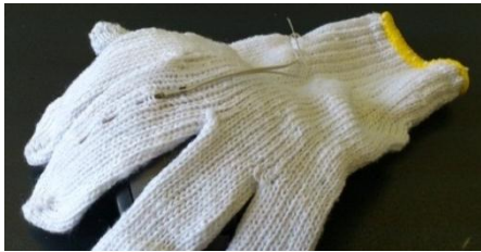
fig.3 IPMC attached to working gloves
