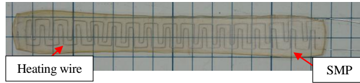
Fig. 3 SMP sheet with embedded electrical heating wire
