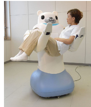
Fig. 1. RIBA lifting a human in its arms.
