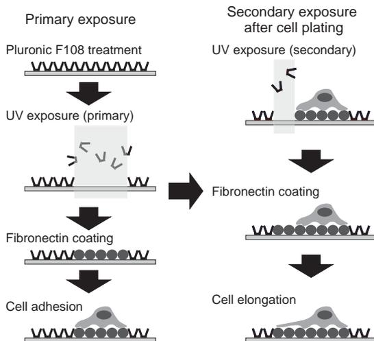
Fig. 1. Fabrication process of caged cell-culturing substrates and cell migration control.
