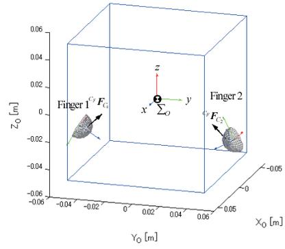
Fig. 7. A rectangular object grasped by two soft-fingers.
