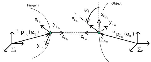
Fig. 5. Contact coordinates before the deformation.
