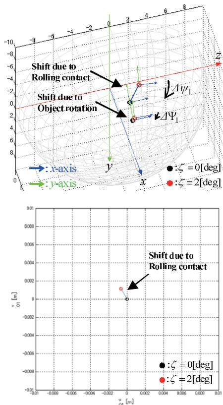
Fig. 13. The changes of the contact configurations on the 1st finger and the object.
